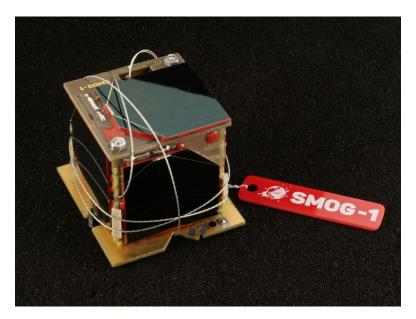
The primary mission of the satellite is the **measurement of electromagnetic pollution generated by human activity** in space around the Earth. This radiation is called electrosmog, from which the name of the satellite is originated. As a secondary mission, a **total ionising dose measurement** system is on board, which measures and studies the effect of solar wind (particles coming from the Sun) on electronics. SMOG-1 has an additional, tertiary
